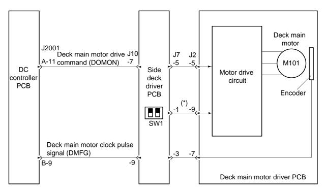
\*Deck main motor high-speed signal (DMHS)
