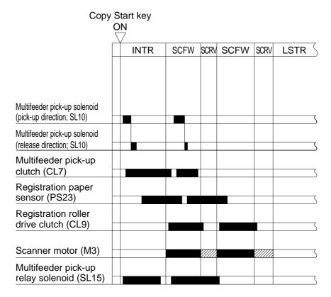
Scanner motor reverse rotation (reverse direction)
