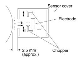
Figure 4-103 Sensor Cross Section
