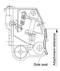
Be sure that the side seal does not protrude inside the cleaner housing.
