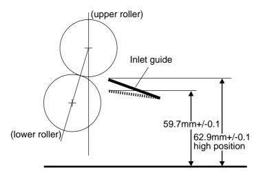
Height of the Fixing Inlet Guide (dimensions indicate center of inlet guide)
