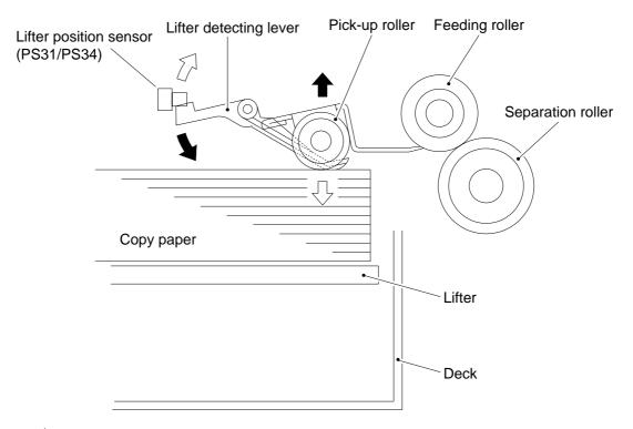
Pick-up roller moves up; the light-blocking plate of the lifter detecting lever lowers to block the lifter position sensor (PS31/PS34).
