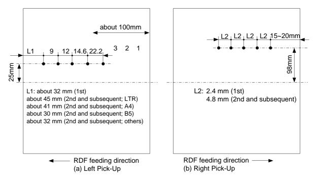
Figure 4-109 Points of Measurement on an Original
