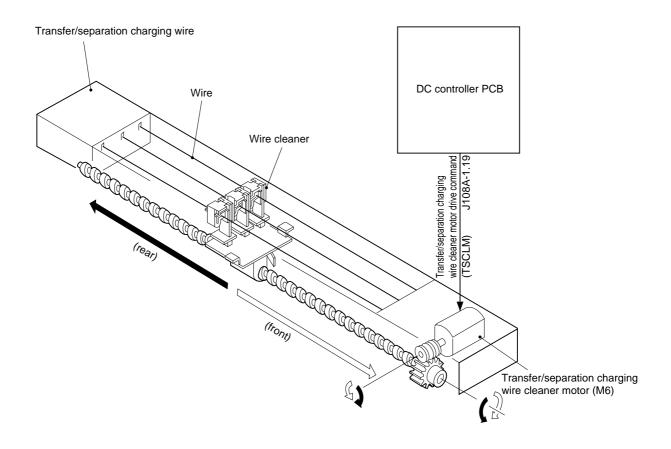
Figure 4-125 (transfer/separation charging assembly)
