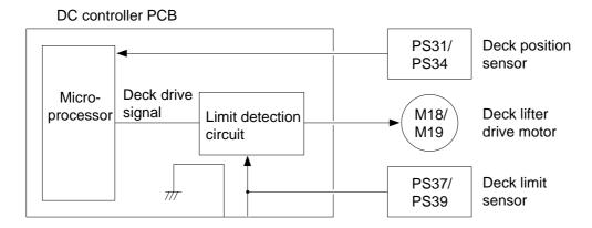
Figure 5-306 Deck Limit Detection (2 cassettes + left/right deck)
